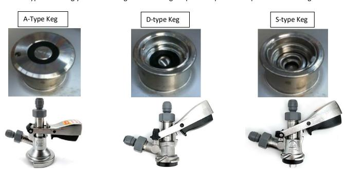
Once you have matched the correct keg coupler to the keg you will need to set up the commercial keg coupler. On a keg coupler there is an inlet for gas and an outlet for liquid. The gas inlet is positioned on a 45-degree angle and the liquid outlet is positioned vertically. It is important to connect the gas line and beer line to the correct inlet and outlet. This is described in the image below.
